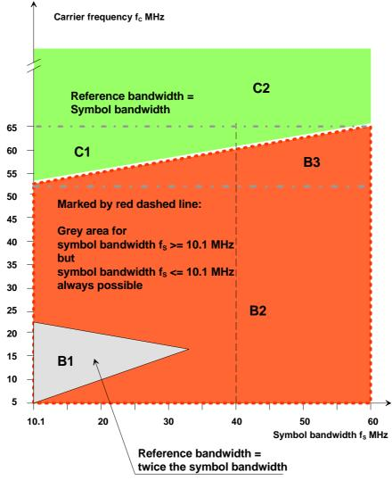
Fig. 12 Ranges B and C:  $f_c$  as a function of  $_s \ge 10.1$  MHz or of the C/N reference bandwidth for white noise with correct C/N display on SFQ
