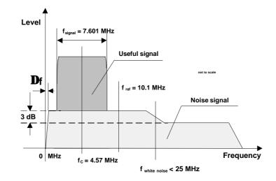
Fig. 13 Signal bandwidth  $f_{\text{signal}}$  as a function of  $f_{\text{c}}$  < 15 MHz for white noise
