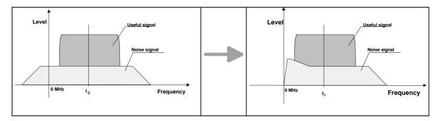
Fig. 3 Frequency reflection about 0 Hz
