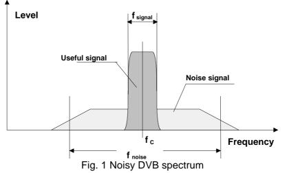
The C/N ratio should, however, be capable of being varied over wide ranges with the aid of a TV test transmitter irrespective of the bandwidth  $f_{signal}$  that is selected. A number of different bandwidths  $f_{signal}$  are used for DVB:
