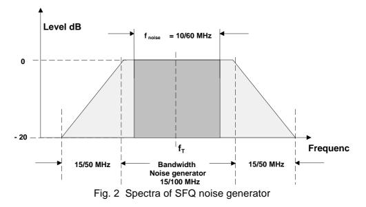
The switchover thresholds between the two bandwidths are at the C/N reference bandwidths  $f_{ref} \geq 10.1$  MHz for a utilized noise bandwidth of 60 MHz and  $f_{ref} \leq 10.0$  MHz for a utilized bandwidth of 10 MHz.
