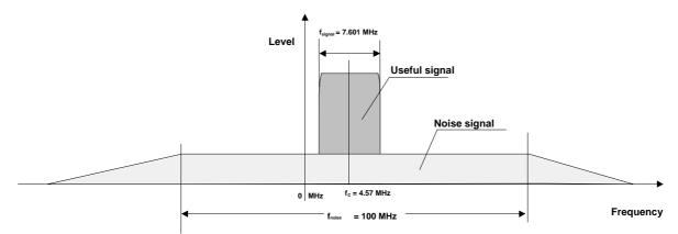
Fig. 8 Non-physical spectrum and broadband noise spectrum
