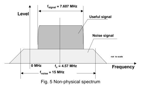
After conversion to the carrier frequency  $f_c = 4.57$  MHz, the spectral components of the 'negative' frequencies are reflected about 0 MHz into the positive range.
