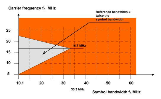
Fig. 11 Carrier frequency 5 MHz <  $f_c$  < 22.5 MHz as a function of symbol bandwidth  $f_s \geq$  10.1 MHz
