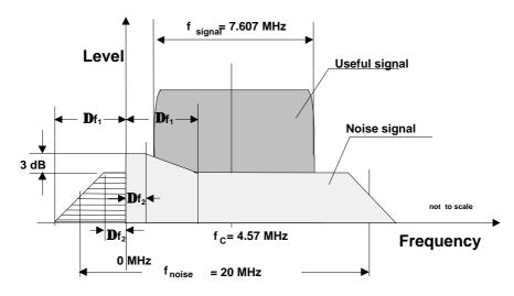
Fig 6 Real spectrum with noise reflection
